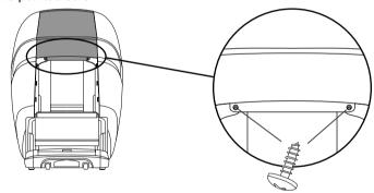
9. Put the back cover-bottom to the right place and align with the four screw holes, then use the flat head screw sleeve top gasket and tighten.
