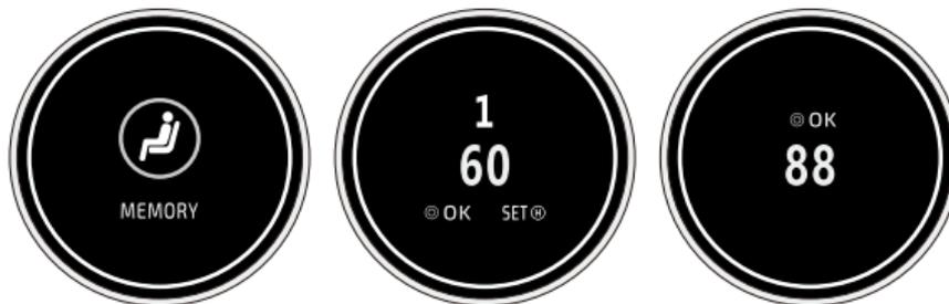
Rotate the knob to MEMORY interface, press the knob once to enter. Rotate the knob to select one position. Press the knob again, and the seat will move to the preset position.
