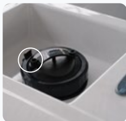
Filter exhaust valve.
